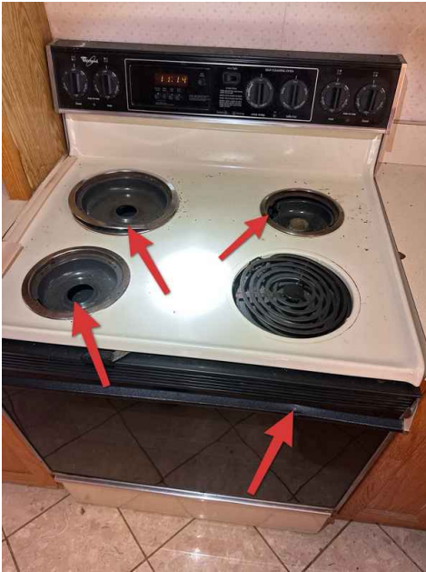
Missing elements and dented handle
